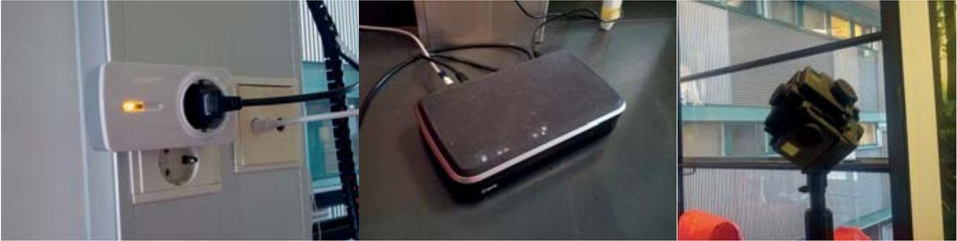
**Figure 2.** Left: Everspring AN158 power meter. Middle: ThereGate router. Right: GoPro Hero 3 Black by Kolor panorama camera.
