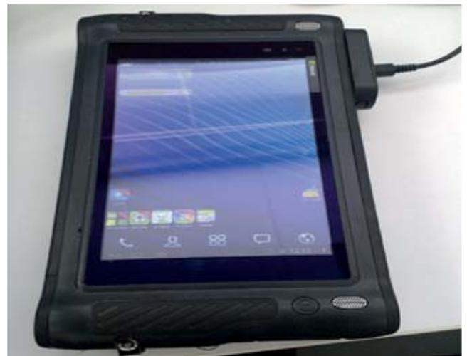
**Figure 3.** Android test device: Elektrobit RaptorPad
