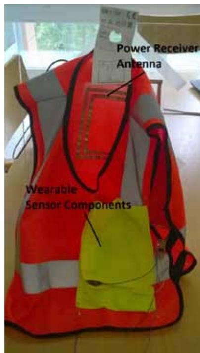
**Acceleration sensors will detect if the child is being pushed, for example. This gives technical means for detecting bullying and intervening with it, while the temperature sensor detects if the child is left out in the cold."**
